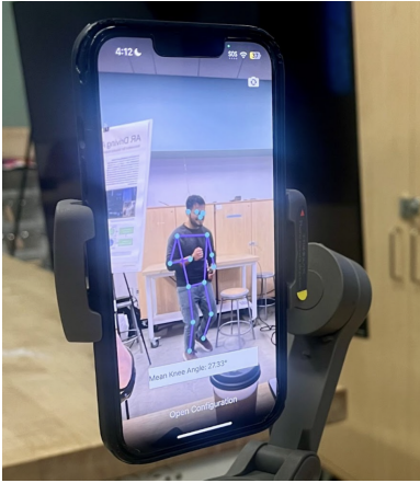
Figure 4. We tested the Non-Visual AR system on 5 participants to evaluate angle detection accuracy and gather qualitative feedback on the user experience.
